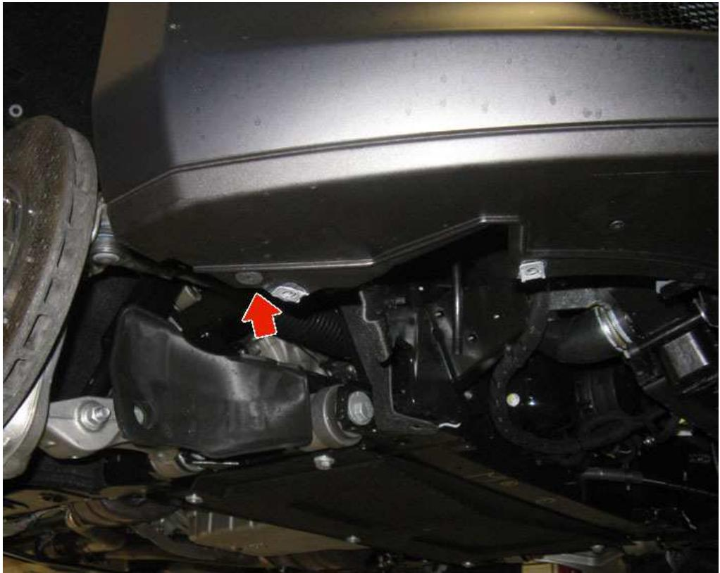
5. Undo the fastening screws on both sides of the mudguard, in the seats of the front light clusters.
