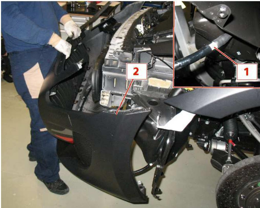
10. When refitting, follow the operations in reverse order, taking care to align the bumper with the mudguard. Also tighten the bumper fastening screws to torque.
